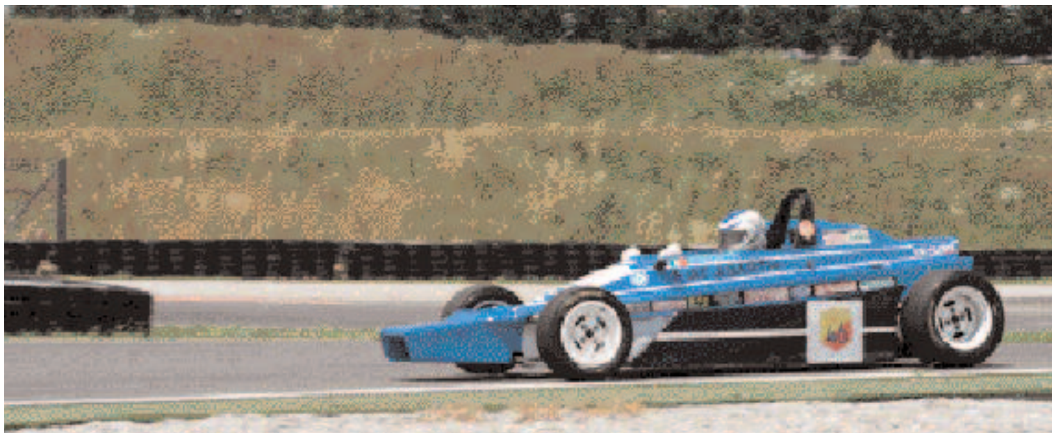
BELOW: Formula Fiat Abarth 033 is a practical track day car powered by a transverse Lancia 2-litre twin-cam power unit
